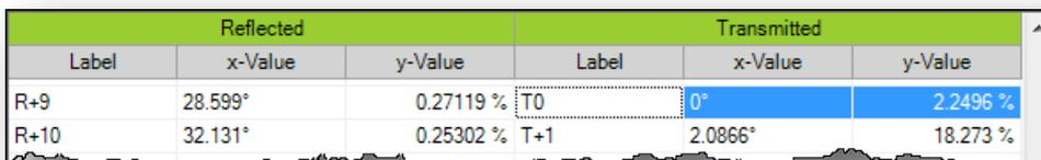
This is a close-up view of the table from the screenshot above, showing the zeroth transmission order (T0) highlighted in blue. The table has columns for "Label", "x-Value", and "y-Value" for both reflected and transmitted orders.
